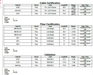
TestDataPro supports both PC and cloud-based options, and come standard with all models of TestPro. Printed test reports for copper and fiber optic include a listed of compliant network support based on the performance of the cable tested. Printed reports are provided for Copper & Fiber certification as well as the combined Multi-Gigabit/PoE Autotest. The Multi-Gigabit/PoE Autotest is a path to a new service offering you can provide to increase your revenue potential.
