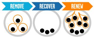
MaxSpace<sup>®</sup> is a no-dig conduit space recovery solution designed to safely remove rigid innerduct from around active fiber cables with little to no load on the cable and no interruption of service. Use that new space to load your conduit with MaxCell and provide the pathways you need now and in the future!
