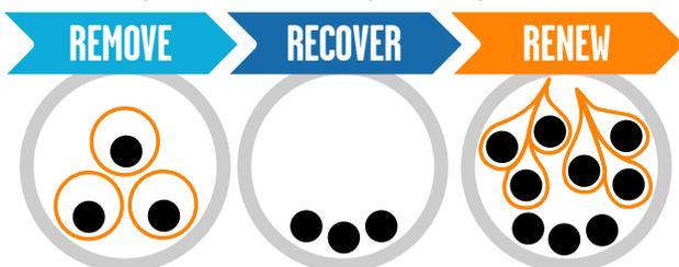
MaxSpace® is a no-dig conduit space recovery solution designed to safely remove rigid innerduct from around active fiber cables with little to no load on the cable and no interruption of service. Use that new space to load your conduit with MaxCell and provide the pathways you need now and in the future!
