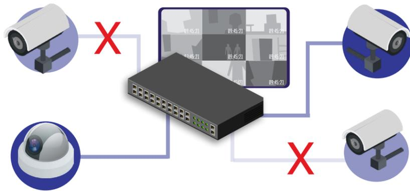
When devices fail or are unresponsive on the network, PoE Watchdog automatically reboots them. These devices are not always within proximity and reduce the need to manually monitor the device status and/or send personnel to go onsite to perform a manual reboot on the unresponsive device(s). This saves you valuable time and money.
