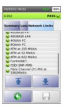
Fig 13: Based on the performance of the cable tested, it is useful to be able to have a detailed view on what network types the link is capable of supporting
