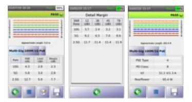
Fig 4: SNR based link speed measurement while under traffic and PoE load
