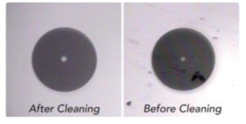
Fig 14: The importance of cleaning the fiber before usage and testing can't be overstated. Dirty fiber can lead to performance degradation. Users should have tools that allow them to see if dirty fiber could be the cause of a performance issue
