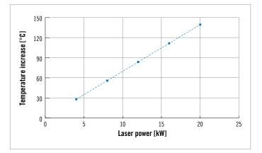
Dependency of the temperature increase of a fused silica piece  $50x 50 \times 20$  mm with an absorption of 80 ppm/cm on the laser power for a beam radius of 0.8 mm.
