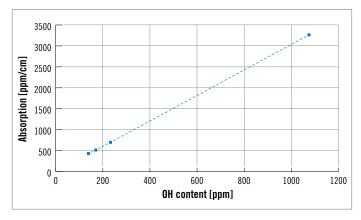
*Correlation of absorption to actual OH content of the measured samples at 946 nm*
