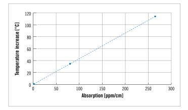
Dependency of the temperature increase on the actual absorption of the simulated fused silica piece, for a 4 kW power beam with 0.4 mm radius.
