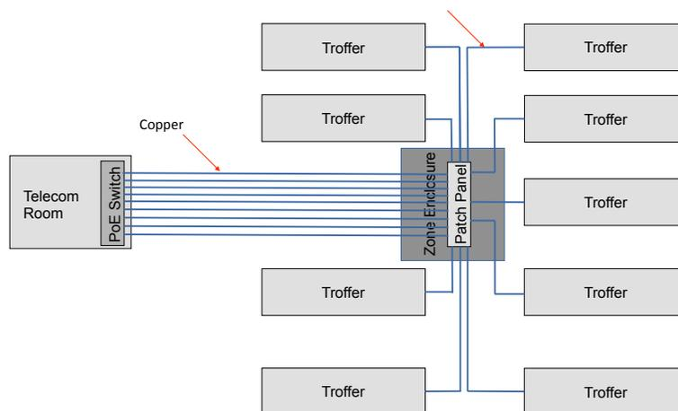
**Figure 1: Centralized PoE switch zone cabling deployment.**
