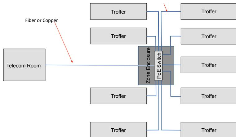
Figure 2: Distributed PoE switch zone cabling deployment.
