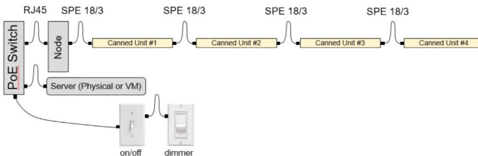
Figure 4: Node-centric architecture.
