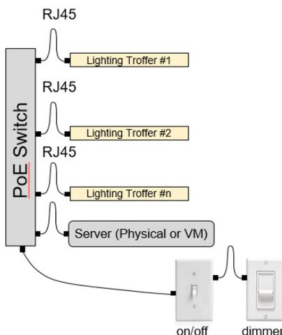
Figure 3: Directly-attached architecture.
