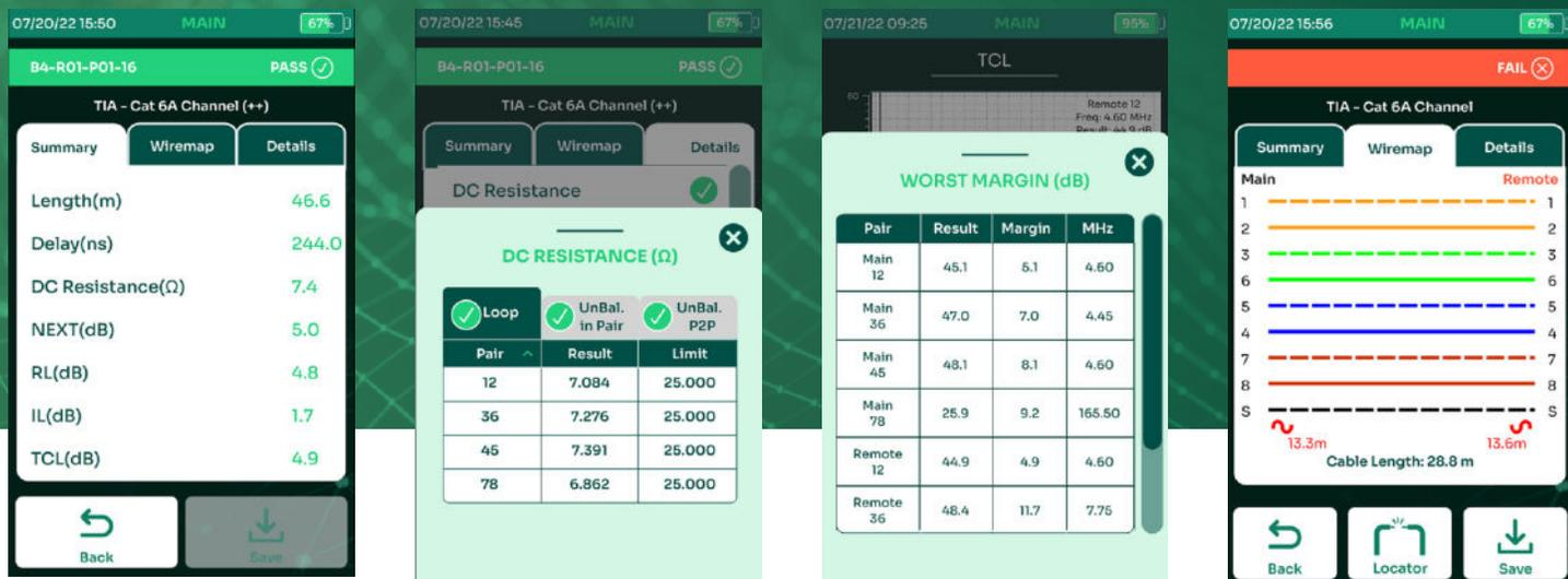
TestPro supports testing and certification for network deployments up to 40 Gigabit Ethernet for Cat 5e, 6, 6A, 7, 8 or Class I/II cabling system. The electrically centered test plug assures the Level 2G/VI accuracy required to support field testing to Cat 8 / Class I/II, and actually exceeds the 2000 MHz requirement, to offer a 3000 MHz platform. As a result, you can feel confident in results over the full frequency range.
