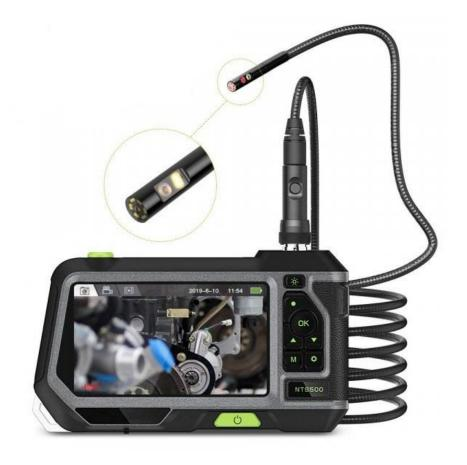
Some bores as well as their enclosures are smaller and may not accommodate an articulating scope. In this case, if a side-facing view is needed, it would be better to consider a dual camera borescope which has two cameras. Dual Cameras allow the advantage of having a front facing camera and another camera on the side which provides a 90 ° angle.
