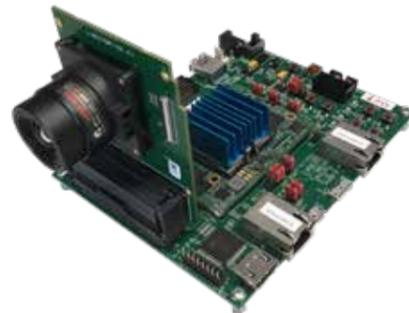
MVDK with MIPI CSI-2 Receiver interface board
