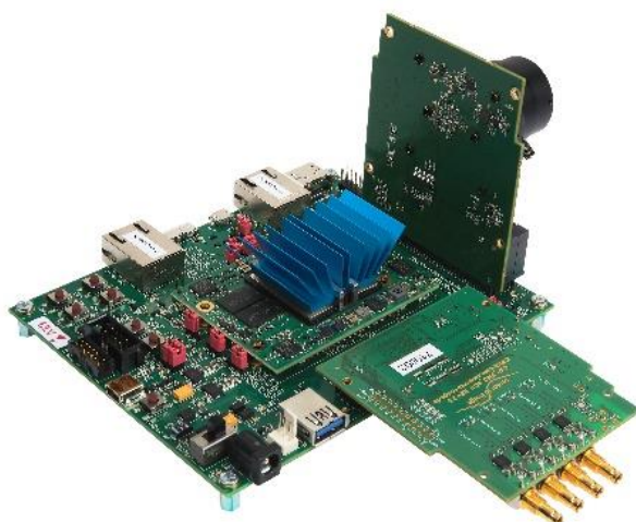
MVDK evaluation board with MIPI CSI-2 sensor and CXP interface board
