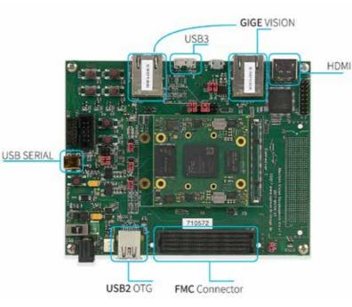
Sensor to Image MVDK (Machine Vision Development Kit) is a hardware platform that eases the evaluation and development of products based on S2I's IP Cores and using any major industrial vision interface. The MVDK base board is highly configurable through the use of FMCs (FPGA Mezzanine Cards). It provides an interface to vision sensors and enables the development of GigE Vision, USB3 Vision and CoaXPress cameras (devices), as well as the design of GigE Vision and CoaXPress hosts.
