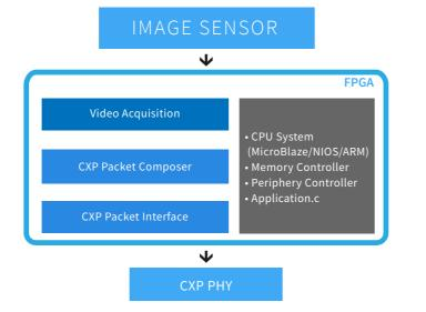
and implements the control channel according to the CXP specification.
