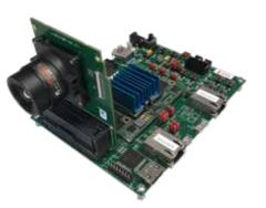
MVDK with MIPI CSI-2 Receiver interface board
